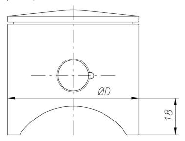
The measure marked on the piston top is the effective one of the piston.
